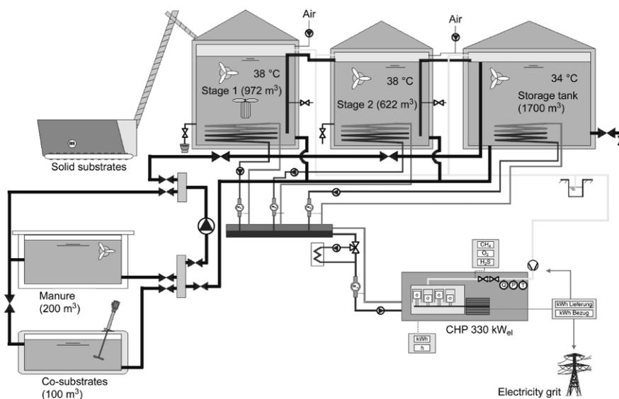
Figure 10. Two-stage biogas plant with gas-tight covered storage tank.
