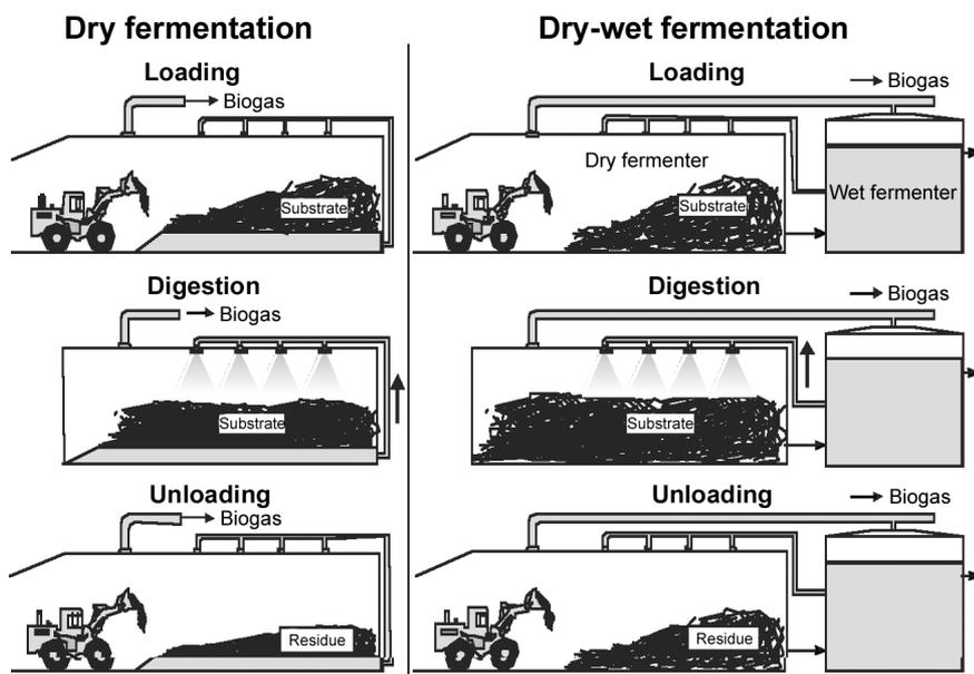
Figure 12. Process variations for dry fermentation in digestion boxes.
