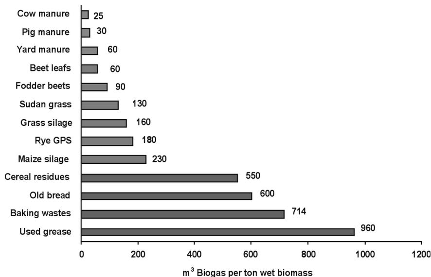
Figure 1. Biogas yield from different substrates.
