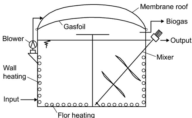
Figure 8. Biogas digester with double membrane roof.
