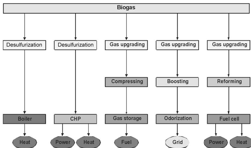
Figure 13. Alternatives for biogas utilization.
