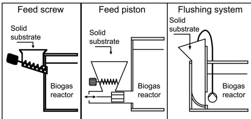
Figure 9. Direct feeding systems for solid wastes and energy crops.
