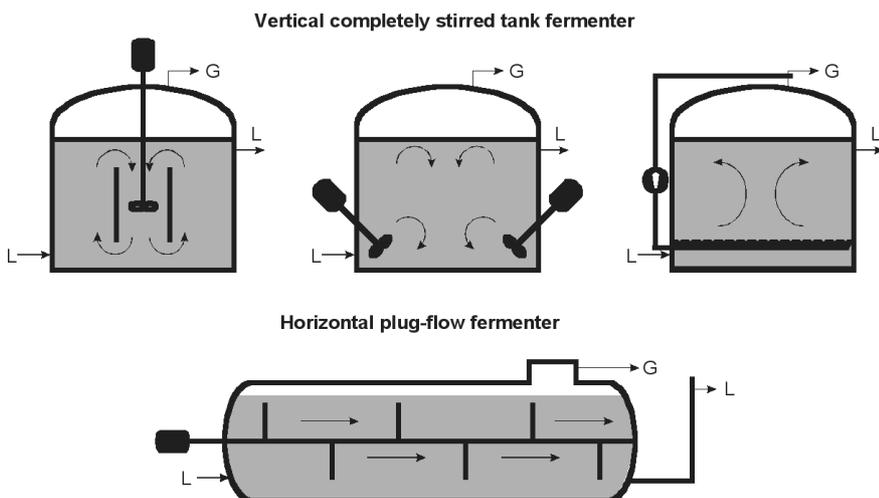
Figure 7. Fermenter types for wet fermentation.
