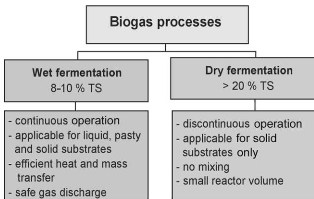
Figure 6. Process alternatives for anaerobic treatment.
